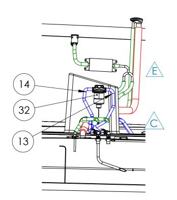
SECTION W-W Fuel filter position SCALE 1:15
